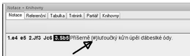
Figure 2: Windows-1250 Code Page in ChessBase. The common Czech letter “z with a hook” is interpreted as the ChessBase “print diagram” code.
