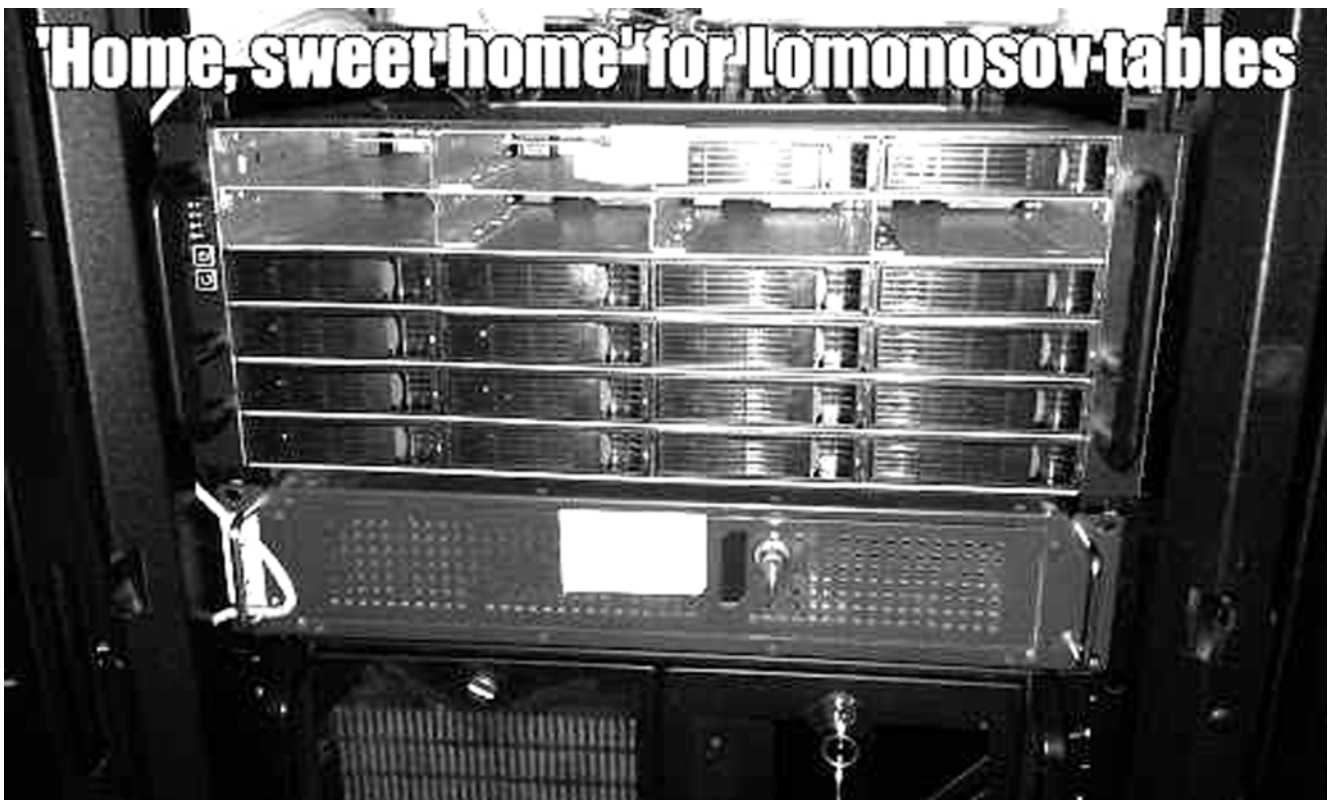
"Home" for Lomonosov tables – in a 24 slot baym 18 hard drives are in use.
